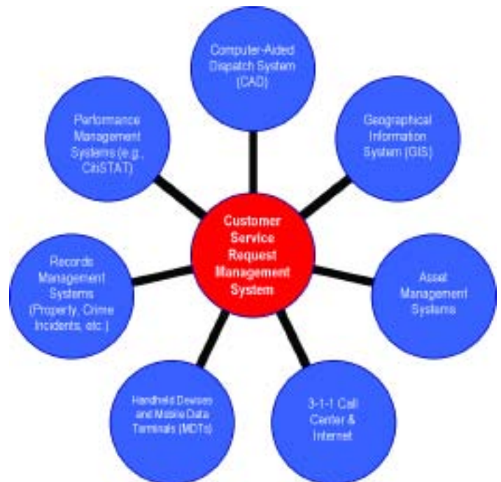
Figure 1.2.1: The CSRM system functions as a hub connecting (and making interoperable) numerous other local government systems and technology-enabled processes that together manage emergencies as well as day-to-day operations.
