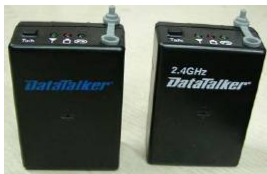
A 900 MHz DataTalker microphone (left) is labeled in blue. A 2.4 GHz microphone is labeled in white.
