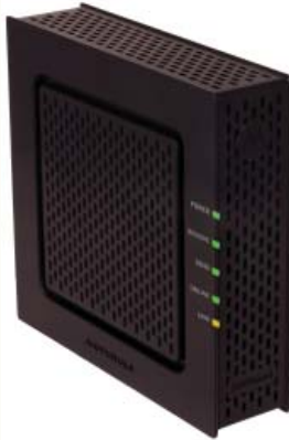
Figure 1: Utilizing the power of DOCSIS 3.0, the SB6120 cable modem enables channel bonding of up to 4 downstream channels and 4 upstream channels: performance which enables operators to offer commercial customers advanced multimedia commercial services with data rates of well over 100 Mbps in each direction.
