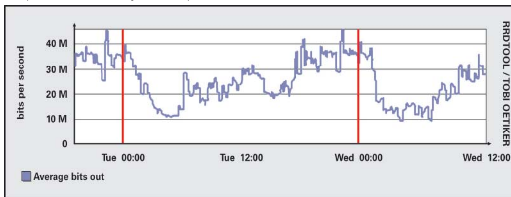
Figure 5: Commercial services can capitalize on usage declines during business hours by allowing MSOs to offer new billable services that are largely consumed between 8 am and 6 pm.
