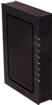
Figure 2: The Motorola SBV6220 DOCSIS 3.0-certified digital voice modem introduces channel bonding into Motorola's digital voice product portfolio. It supports the full range of DOCSIS 3.0 features, including IPv6 and Advanced Encryption Services.
