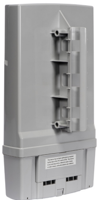
Easy to use mounting bracket on the back of the CPEo 450.
