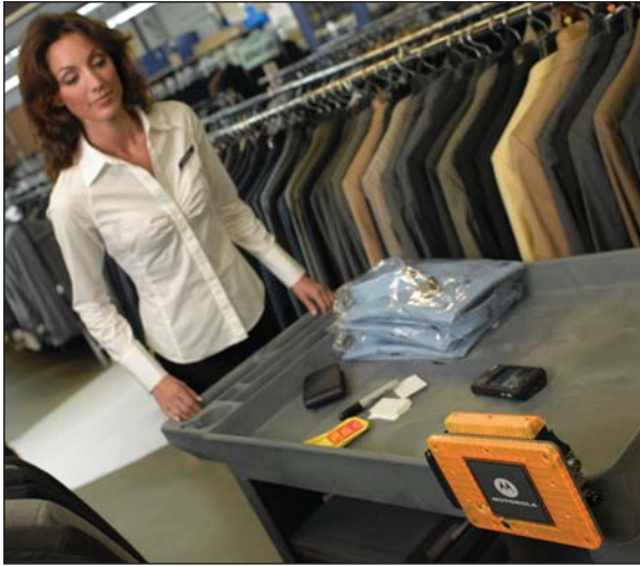
A rolling cart equipped with an RFID reader can make daily cycle counts of tagged merchandise practical.
