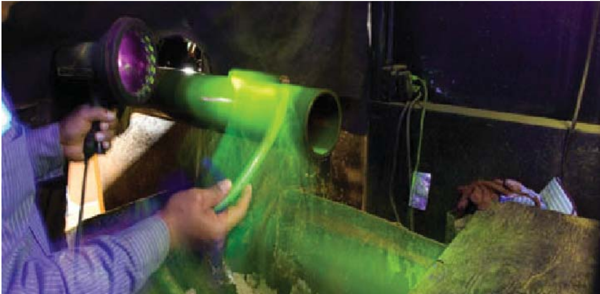
picture 3: Special-End-Area Inspection
