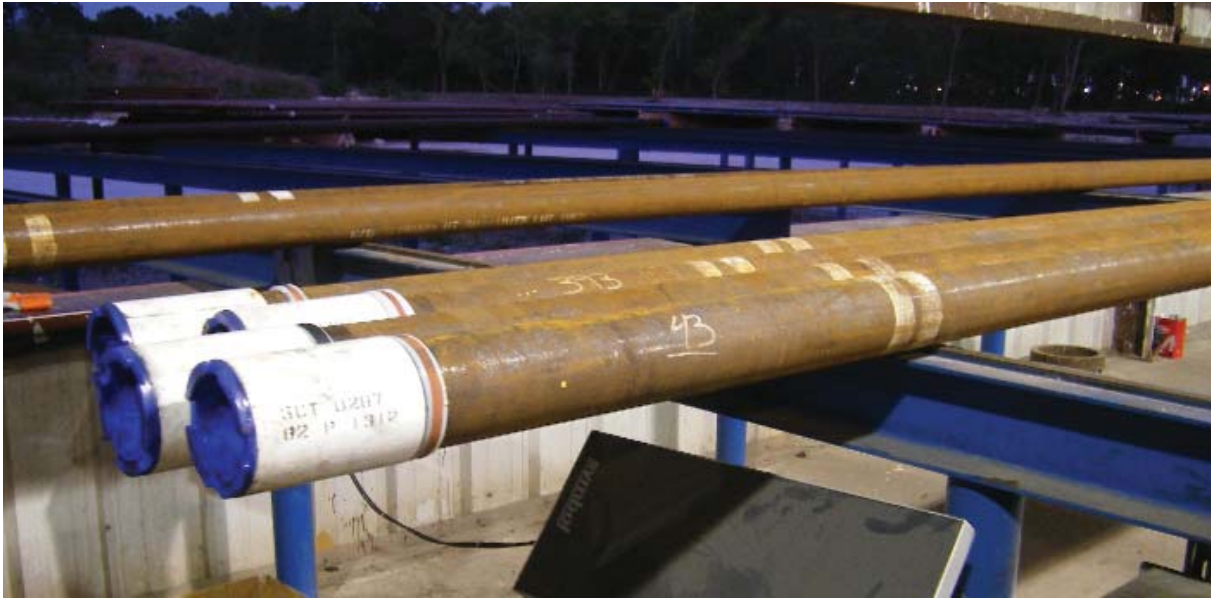
picture 5: Outgoing Electro-Magnetic Inspection (RFID Read)
