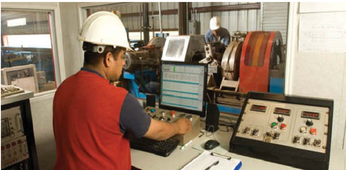
picture 4: Electromagnetic Inspection
