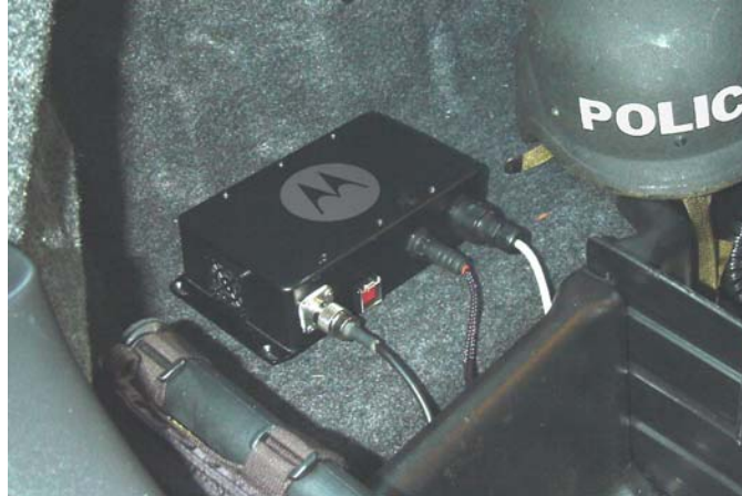
Figure 2-2. VMM6300 Trunk Mounting
