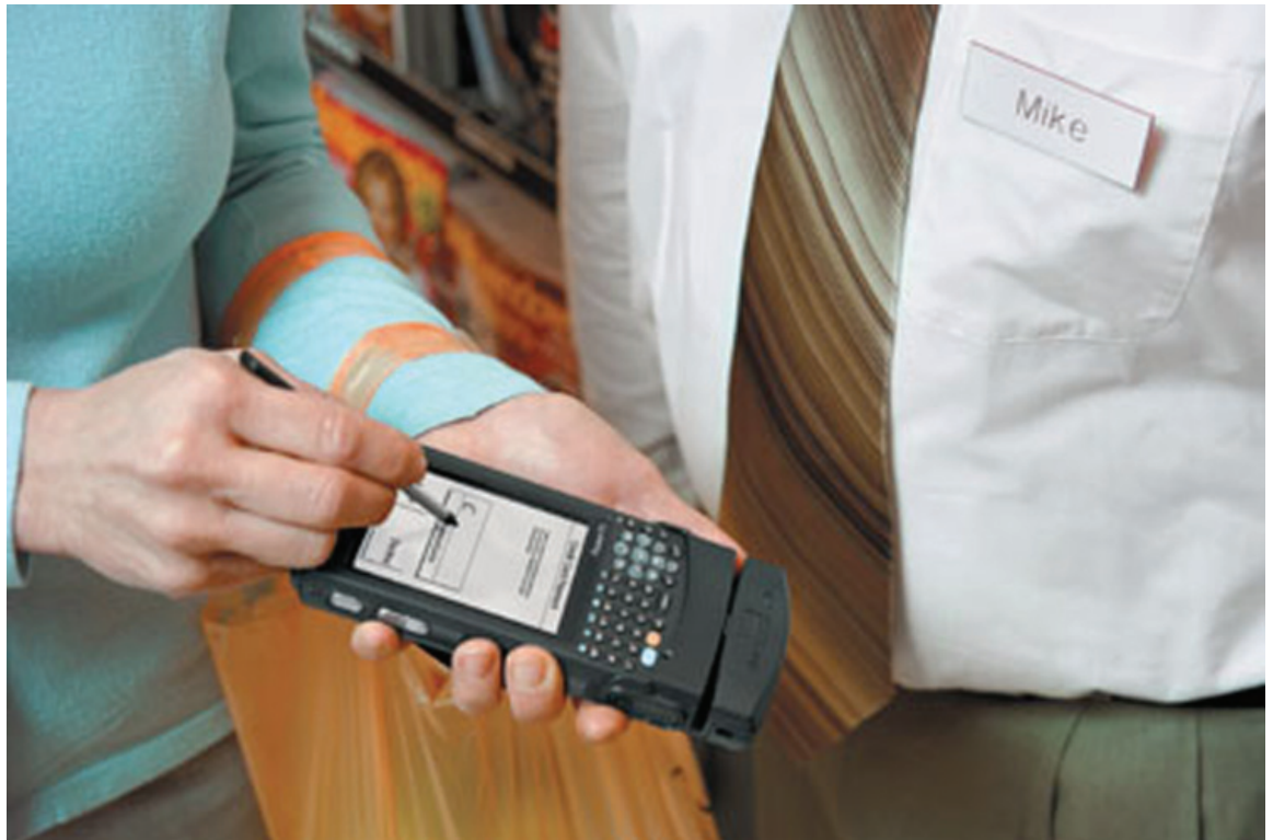
Using signature capture at the point of sale, electronic receipts and signatures are stored online, which can dramatically decrease the time and costs associated with receipt retrievals and related charge backs.
